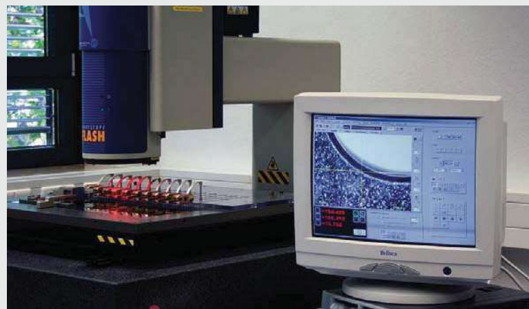
Optical coordinate measuring machine (3D): Optical 3-coordinate measurement, measurement precision down to 3 µm and serial measurement possible. Contact-less measurement system for determining diameters, radii, angles etc.
