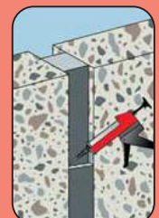
Optional: Wipe with sealing compound after expansion of the tape.
