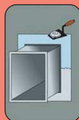
Apply fire-retardant cement. Board up larger ducts on one side.
