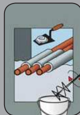
Mix and apply fire-protection cement.
