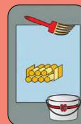
Insert mineral fibreboards. Finally, coat the partition surface, the cables and the cable-support systems with fire-retardant coating (at least 1 mm thick).
