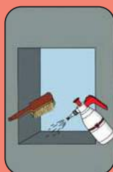
Clean opening and moisten reveal.
