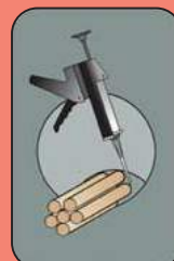
Affix fire protection plugs on both sides of the wall and fill remaining gap and spaces between cables with SUS 1 Fire Protection Putty.
