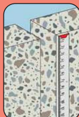
Measure joint and cut tape to proper size.
