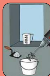
Premix dry cement. First put water, then cement into the mixing container. Mix for 4 minutes at 300 to 400 rpm.
